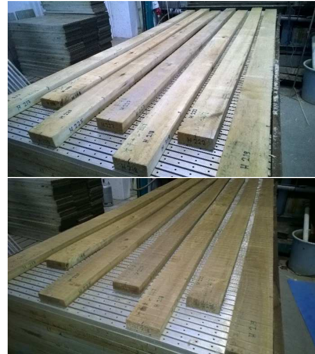
A set of boards ( 40 \times 100 \times 2,700 \text{ mm}^3 ) before and after the modification. Figures: Nextimber Ltd.
